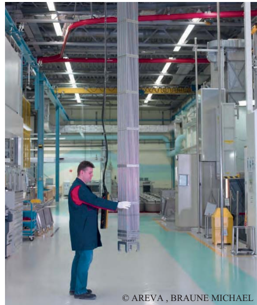
Fig. 4: Pressurized water reactor assembly at the fuel fabrication plant in Lingen, Germany.
