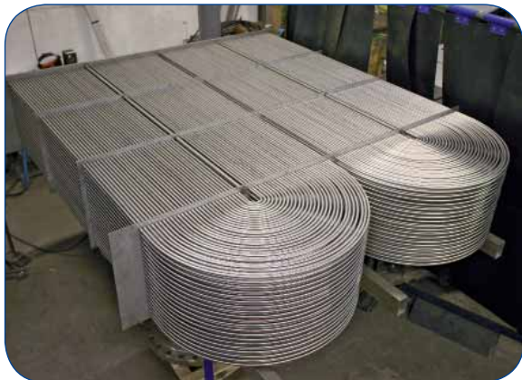
Fuel Pool Cooler
